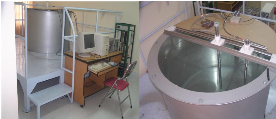
Figure 1. Multi-function water-filled Howitzer using an isotope neutron source was made in the Nuclear Research Institute.
